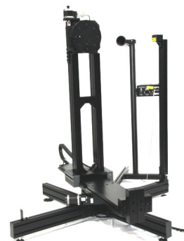
Fig 1. SSL-10-150-30 goniometer with an alignment laser and stray light tube.
