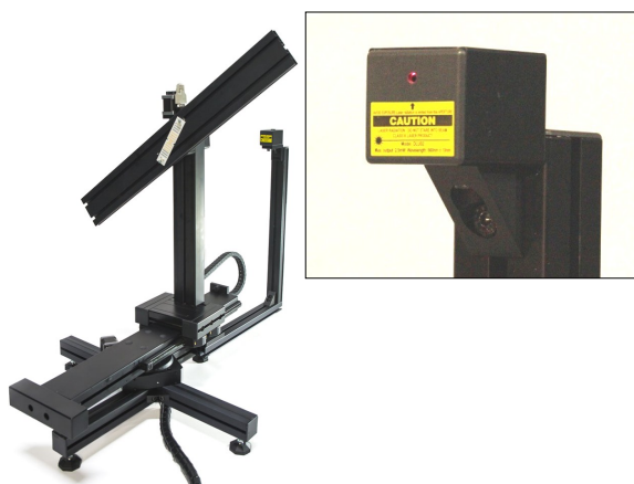
Fig 2. SSL-6-70-20 Goniometer. The alignment laser helps aligning the Luminaire onto the optical axis and also useful in setuping the goni and photometer into the same optical axis in a e.g. new lab.
