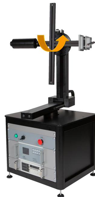
Fig 11. Measurement setup of burning position effect in case of SSL G-900R goniometer.
