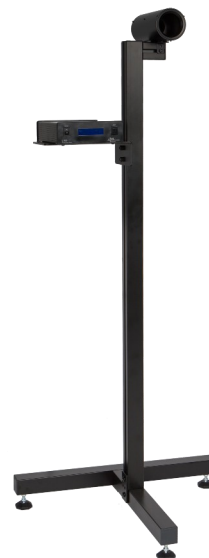
Fig 4. The stray light tube and stand for a photodetector.
