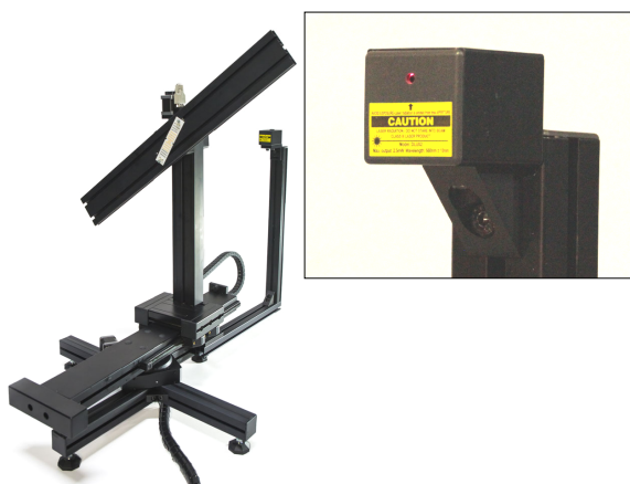
Fig 2. SSL-6-70-20 Goniometer. The alignment laser helps aligning the Luminaire onto the optical axis and also useful in setting up the goni and photometer into the same optical axis in a e.g. new lab.
