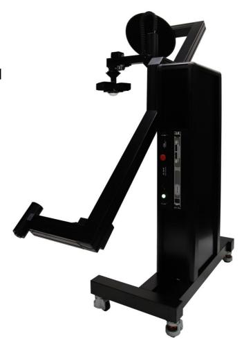
Optimal for testing luminaires with a luminous area of smaller than 270 mm.
