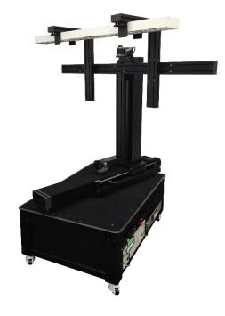
Fig. 3. SSL BPC-C setup in nominal burning position  $(E_{nomBP})$  of linear light source. (photo: SSL LUMI 180 goniometer).
