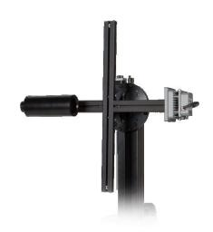
Fig. 2. SSL BPC-C. The burning position corrector setup at normalized measurement position ( $E_{measBP}$ ) in case of type C goniometer (photo: SSL LUMI 90 goniometer).
