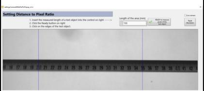
The distance scale of the image can be calibrated by a Define mm/pixel —button. The diameter of circle can be user-defined and its coordinates is chosen by mouse-clicking.
