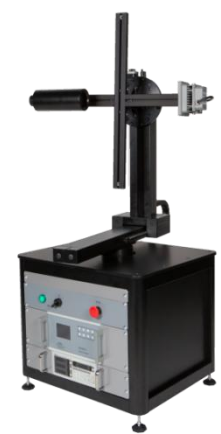
Burning Position Correction Setup for C type (photo: SSL LUMI 90)
