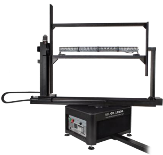
B Type Measurement for Automotive Lights (photo: SSL LUMI 120)
